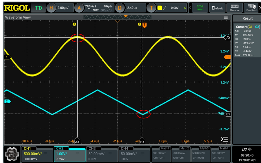
Figure 10.13 Track Measurement (after Horizontal Expansion)
